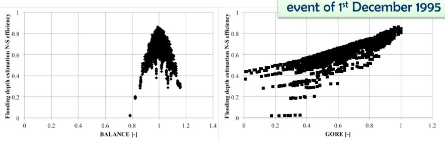
BALANCE is higher sentitive: rainfall depth has a major impact on flooding; a wrong estimation of rainfall can impact negatively on model performance
