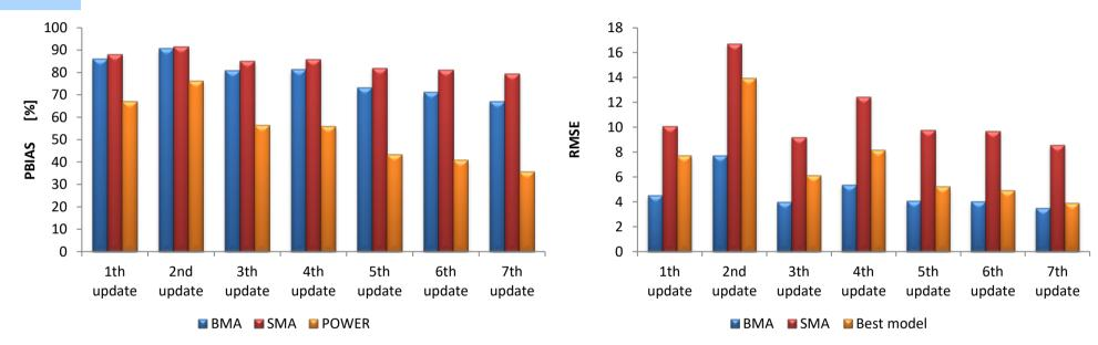
BMA predictions are better than that of the SMA and of best individual predictions in terms of RSME BMA PBIAS and RMSE are less than SMA ones The improvement in terms of uncertainty reduction by BMA is around 10% with respect to the best individual model
