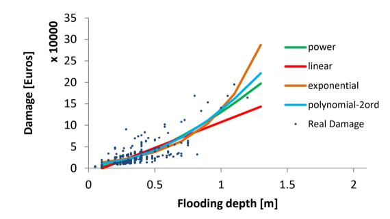
Flooding data are often piecemeal, affected by measuring errors and spatially aggregated. In consequence, the flood damage assessment is usually affected by a degree of intrinsic uncertainty that cannot be realistically eliminated
