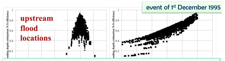
Better rainfall knowledge generally means a better estimation of flood depth but the uncertainty related to rainfall knowledge is still high: GORE values equal to 0.8 can produce N-S flooding estimation criterion ranging from 0.5 to 0.75
